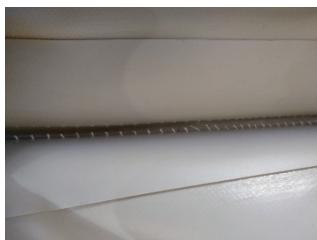
When you have inflated the driving tubes you will see a split seam. This seam is not a defect but a so-called fixation seam, which is set during the production process so that the connecting bottom can be glued at right angles to the two driving hoses. When inflating, this fixation seam opens up and the separated stitch threads can be seen, which rub away over time.
