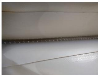
When you have inflated the driving tubes you will see a split seam. This seam is not a defect but a so-called fixation seam, which is set during the production process so that the connecting bottom can be glued at right angles to the two driving hoses. When inflating, this fixation seam opens up and the separated stitch threads can be seen, which rub away over time.
