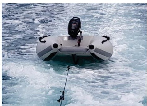
Only the two rings at the bow (the two fixing rings under the floor at the bow) are used for towing. The optimal solution would be to glue two large towing rings at the bow under the connecting floor. When towing, it is essential to ensure smooth throttle changes. Rough jerky throttle changes can cause damage. The transom tubes must never be used as towing brackets.
